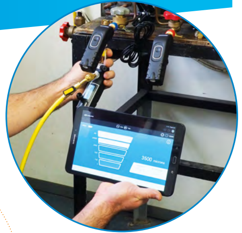
MEASURE EVACUATION WITH THE SI-RV3 VACUUM PROBE
