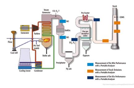
Many power plants use CEMS (Continuous Emissions Monitors) to analyze the total emissions being released from the stack of the power boiler. This information alone is not sufficient to pinpoint any deficiencies in the De-NOx system.
