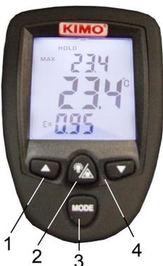
1 - Up button. It allows to increment emissivity and high and low alarm thresholds and to go to the following recorded value. It also allows to navigate between MAX, MIN, AVG and LOG.
