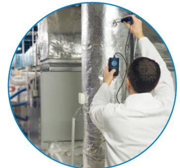
TEMPÉRATURE, VITESSE ET DÉBIT D'AIR DANS UN CONDUIT
