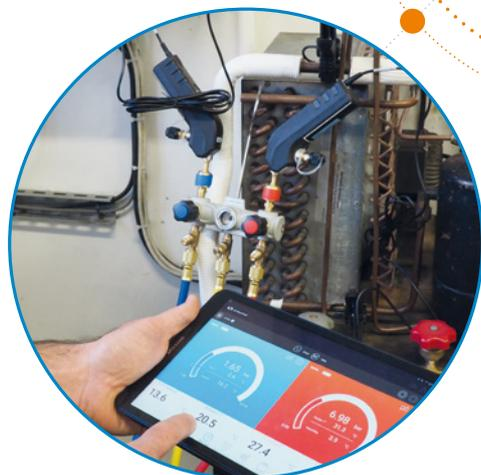
CONTRÔLE AVEC MANIFOLD
