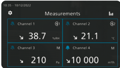
Trend indicator: up to 4 parameters displayed simultaneously
