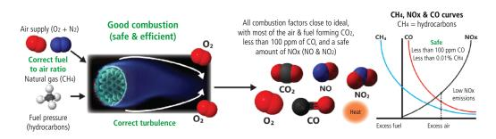
However, in the case of Burner Malfunction, CxHy and CO levels often rise indicating decreased combustion efficiency and overall safety, while increasing cost of production.
