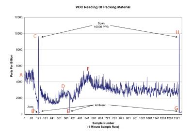
The graph below displays and proves the accuracy the unit holds. The beginning of the test (labeled by point A) captures the higher levels of VOCs released from the opening of bag packing peanuts. The monitor was able to capture the VOC readings rising toward levels of 4,000-6,000 parts per billion. The monitor was then brought outdoors to clean ambient air (at point B) where the VOC levels quickly dropped, and the readings reflected the new cleaner environment.
